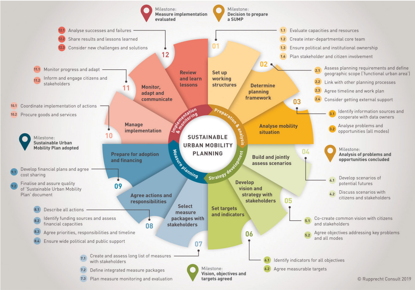
Figure 15: The SUMP cycle and its different phases (= four quadrants) and steps (12 = segments). © Rupprecht Consult.
